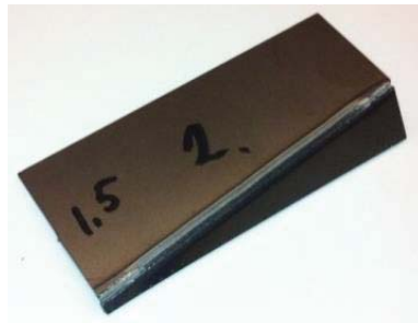
Figure 7 – Specimen used for hot crack susceptibility test according to E SEP 1220-3.
