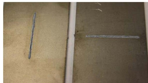
Figure 14. Showing a non-deformed 1.5 mm sheet from a cross-tension test. The failure is in the interface.
