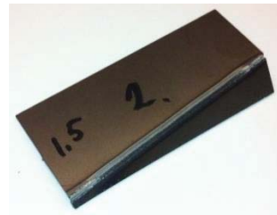
Figure 17. Showing the bended sample. The bend is done along the seam showing the oxidized length of the crack.
