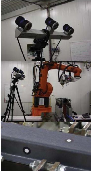
Figure 4 The camera (top), set-up (middle) and measurement points (bottom) used for measurement of distortions during welding.
