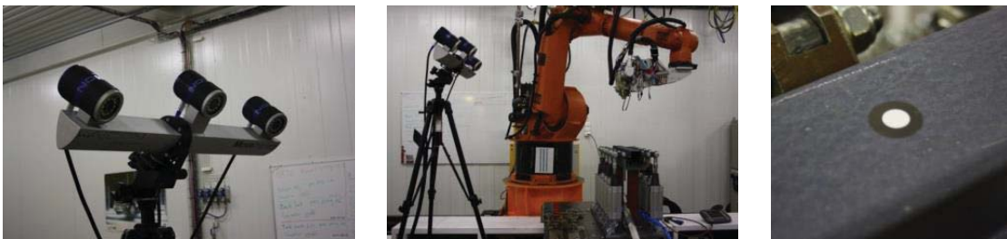
Figure 8 – The optical measurement system used for recording of distortions. The system recognizes measurement points (small circular stickers) placed on the component, and record the position with x-, y-, and z- coordinates at a frequency of 1-6 Hz.
