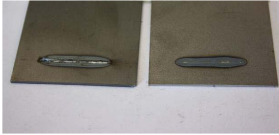
Figure 15. Showing the not fully penetrated 1.5 mm sheet (left = top, right = bottom).
